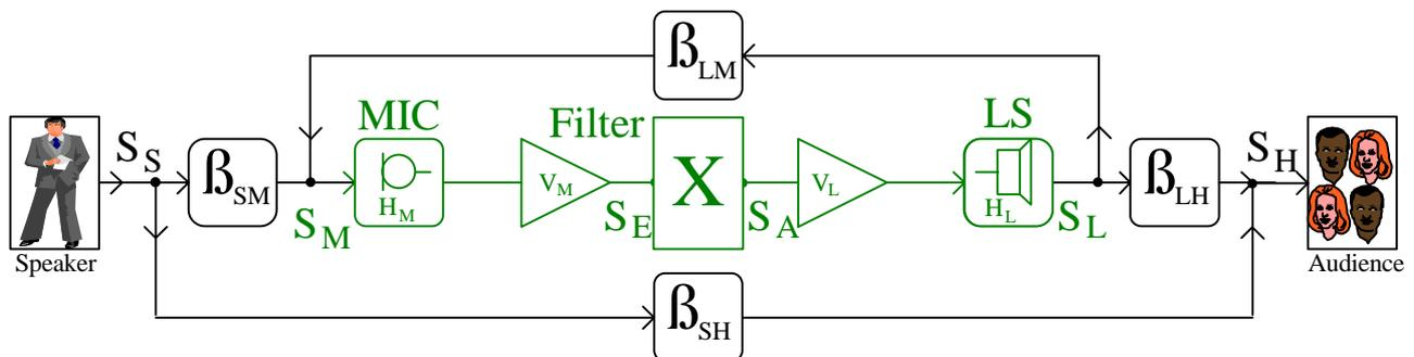
Fig. 1 Block diagram of a simple sound system including filter  $X$
