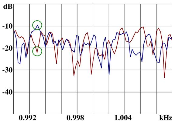
Fig. 6 Increased part of the transfer function for two different microphone positions
