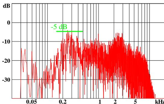
Fig. 4b Loop gain with subtraction filter
