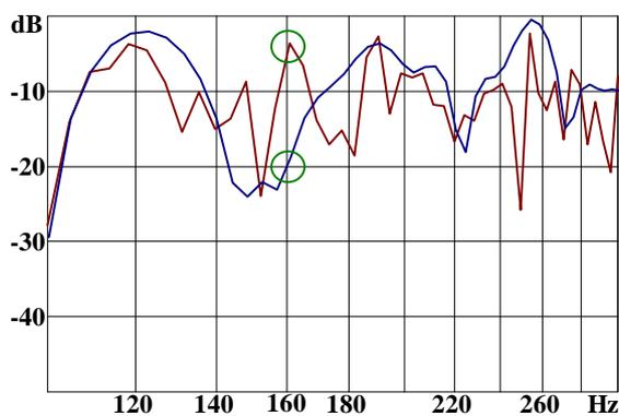
Fig. 7 Increased part of a transfer function and the accompanying adaptive filter function (60 ms filter length)
