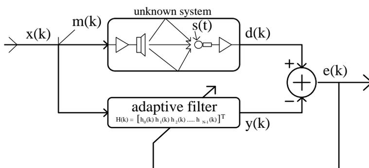
Fig. 5 Block diagram of an adaptive FIR filter
