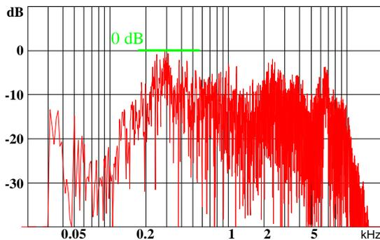
Fig. 4a Loop gain without filter
