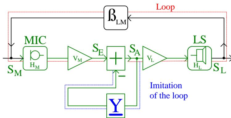
Fig. 2 Loop with subtraction filter
